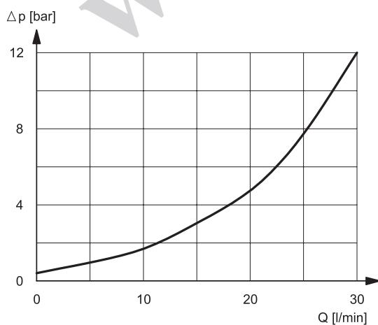
Pressure drop with free flow B→A through check valve.
