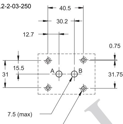
NOTE: The RPCED1 mounting interface, with CETOP 03 holes, must not have P and T ports or must have the 0113388 subplate (to be ordered separately)
